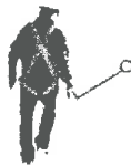
Fall FACTOR 1 anchor point located at the same level of the back anchor point of the harness
